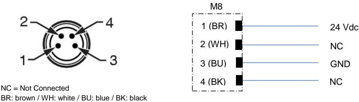
Figure 3 – Wiring instructions (M8 – Power supply connector)
