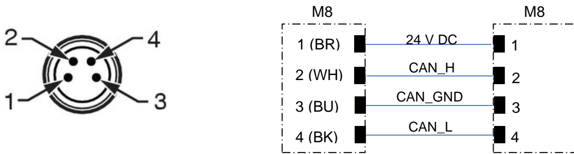
Figure 4 – Wiring instructions (M8 – Coval bus connector)
