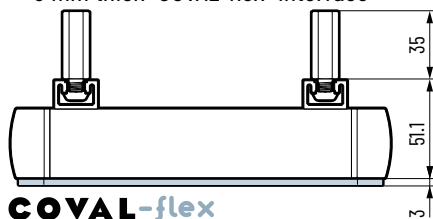
3 mm thick "COVAL-flex" interface
