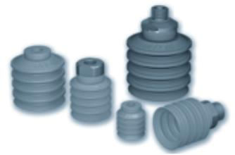
The MVP series suction cups are designed to the handling of raw food or flexible packaging at high speeds. The thin gripping lip allows to fit with the product to be handled and the 4.5 bellows give a swivelling effect to ensure the positioning of the suction cup when the product is held. Furthermore, once in grip, the rigidity of the compressed bellows ensures a very good prehension of the object and avoids the swing effect.
